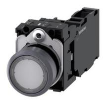
Illuminated pushbutton, 22 mm, round, plastic with metal front ring, clear, pushbutton, flat, momentary contact type, with holder, 1 NO+1 NC, LED module with integrated LED 110 V AC, screw terminal, with laser labeling, symbol number according to, ISO 7000 or IEC 60417
