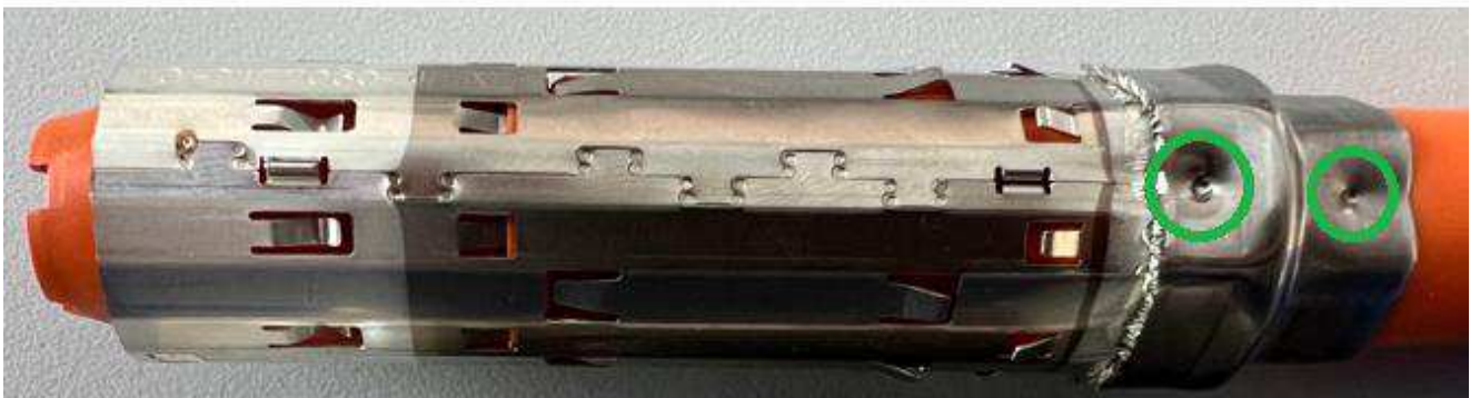
OK crimp – dents – All dents are present with correct depth.
