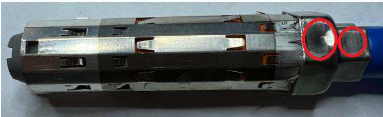
NOK crimp – dents – Dents on cable side are completely missing. Dents on shield side are present but with insufficient depth.
