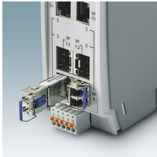
Figure 3-10 Inserting the SFP modules (example)
