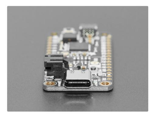
Inside the RP2040 is a 'permanent ROM' USB UF2 bootloader . What that means is when you want to
