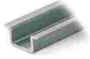
Item no.: 210-118 Steel carrier rail; 35 x 15 mm; 2.3 mm thick; 2 m long; unslotted; according to EN 60715; silver-colored
