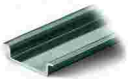
Item no.: 210-113 Steel carrier rail; 35 x 7.5 mm; 1 mm thick; 2 m long; unslotted; according to EN 60715; silver-colored
