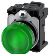
Indicator light, 22 mm, round, metal, shiny, green, lens, smooth, with holder, LED module with integrated LED 24 V AC/DC, spring-type terminal, with laser labeling, upper case and lower case, always upper case at beginning of line
