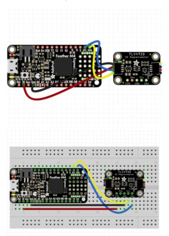
Board 3V to sensor VIN (red wire)
