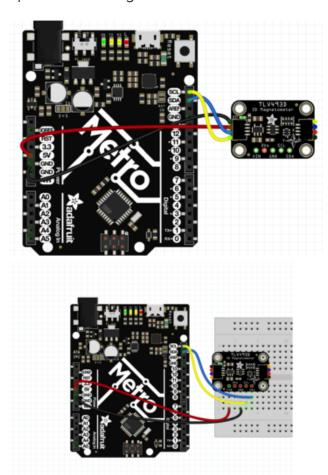
Connect board VCC (red wire) to Arduino 5V if you are running a 5V board Arduino (Uno, etc.). If your board is 3V, connect to that instead.
