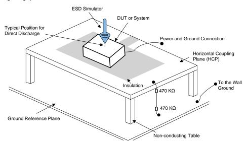
Figure 2. System Level ESD Test Setup
