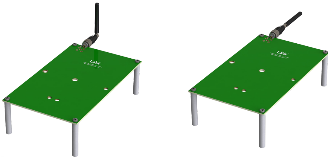
On edge of ground plane, bent 90 degrees
