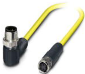
Sensor/actuator cable, 4-position, PVC, yellow, shielded, Plug angled M12 SPEEDCON, A-coded, on Socket straight M8, cable length: 0.5 m
