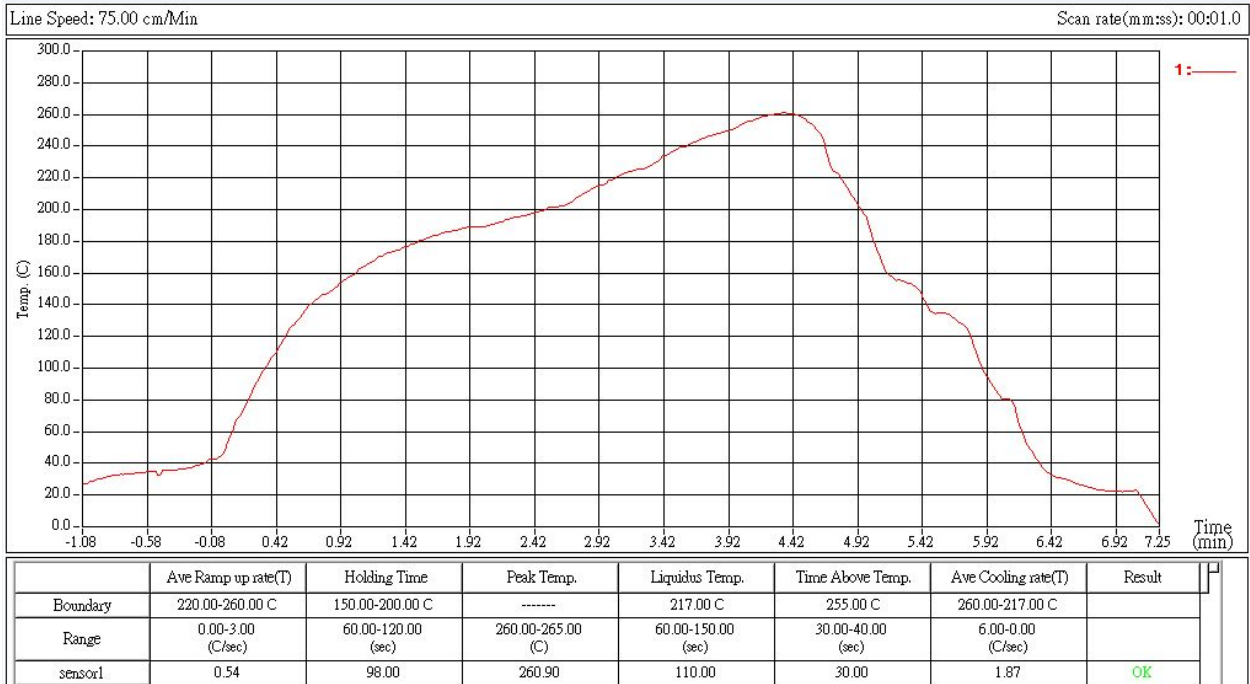
Figure 8.3 Solder Reflow Profile
