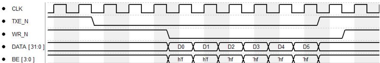
Figure 4.3 245 Synchronous FIFO mode bus master write cycle
