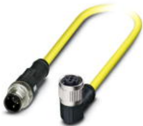
Sensor/actuator cable, 3-position, PVC, yellow, Plug straight M12 SPEEDCON, A-coded, on Socket angled M12 SPEEDCON, A-coded, cable length: 1.5 m
