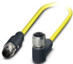
Sensor/actuator cable, 3-position, PVC, yellow, shielded, Plug straight M12 SPEEDCON, A-coded, on Socket angled M12 SPEEDCON, A-coded, cable length: 1.5 m
