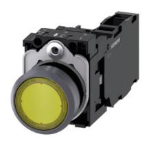
Illuminated pushbutton, 22 mm, round, plastic with metal front ring, yellow, pushbutton, flat, momentary contact type, with holder, 1 NO+1 NC, LED module with integrated LED 230 V AC, screw terminal, with laser labeling, lower case
