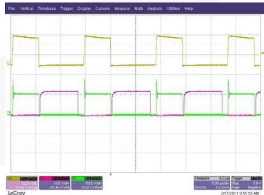
Figure 7. FAN6754AMR+FAN6204MY, 115V/60Hz, 80% Load (Ch1: Gate, Ch2: Gate_SR, Ch4: V d5 )
