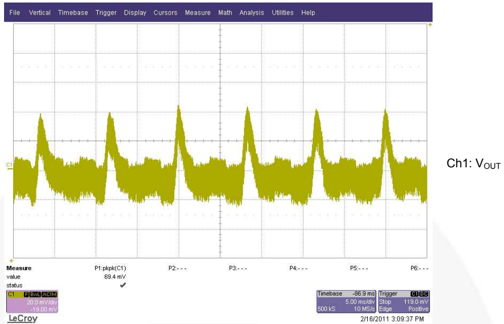
Figure 2. 90V / 60Hz at Maximum Load
