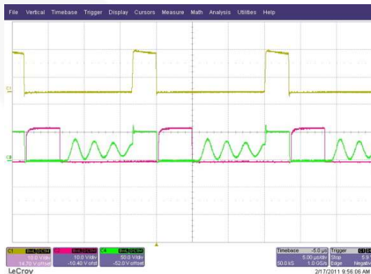
Figure 6. FAN6754AMR+FAN6204MY 115V/60Hz, 20% Load (Ch1: Gate, Ch2: Gate_SR, Ch4: V d5 )
