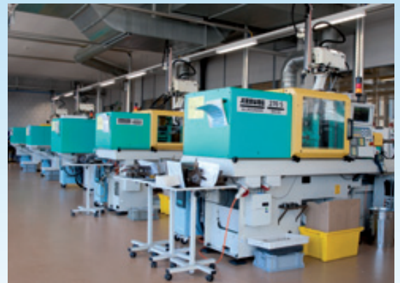
Injection of insulators
