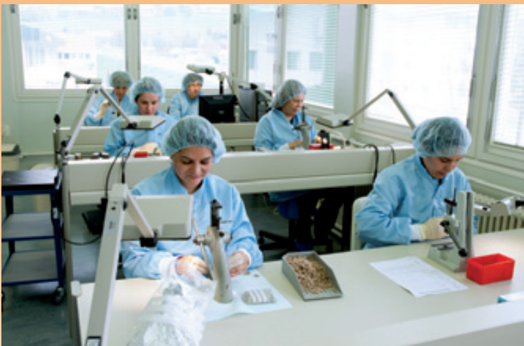
Clean room, assembly of fibre optic contacts
