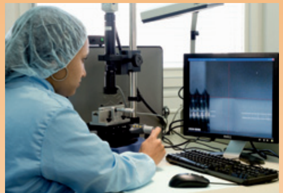
Clean room, inspection of fibre optic assembly
