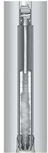
Vapor quenches arc at first current zero
