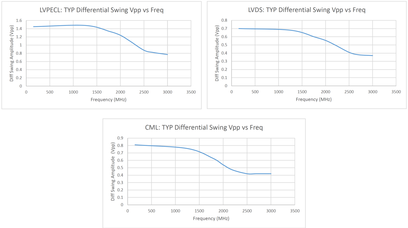
Figure 2.1. Typical Clock Output Swing Amplitudes vs. Frequency
