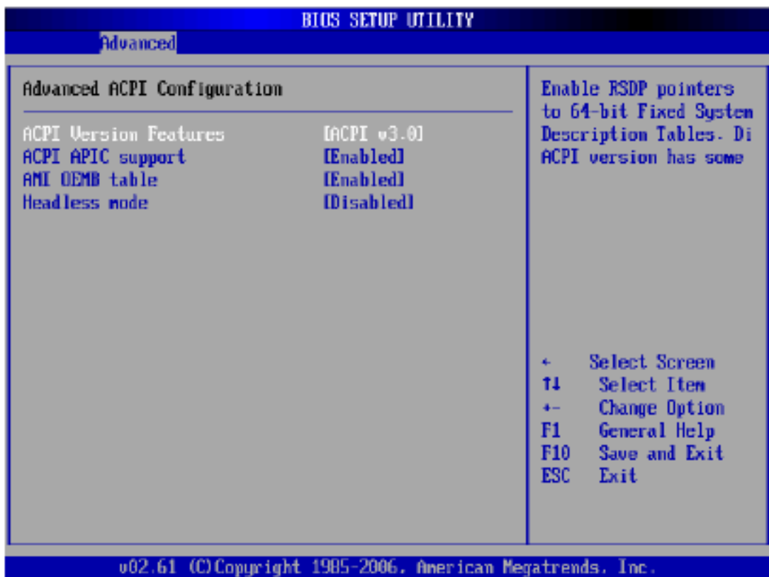
Figure 4.11: Advanced ACPI Configuration
