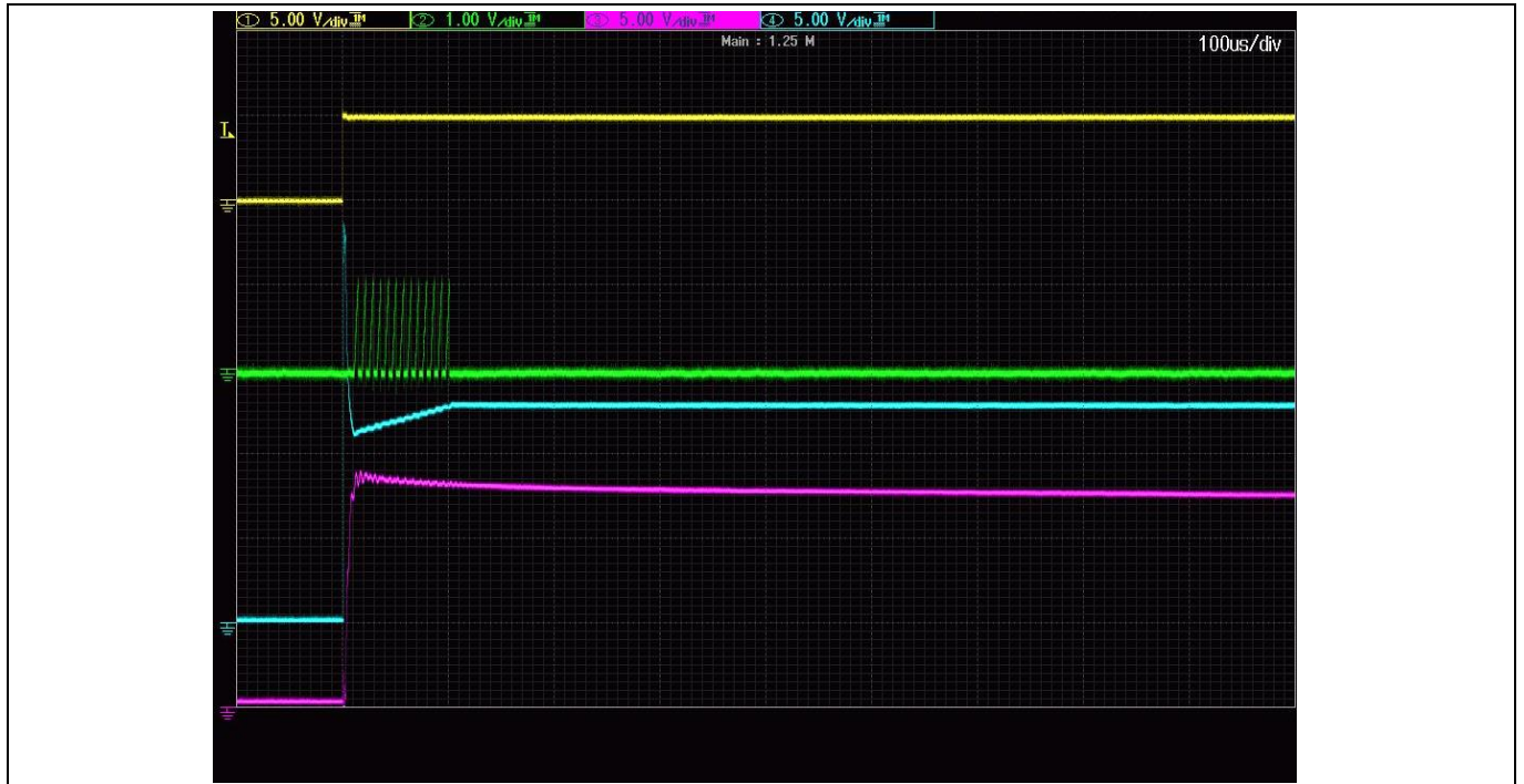
Figure 3 Waveforms from OFF to ON mode [Yellow V_{IN} ; Green V_{RS} ; Blue V_{GS(AUIR3241S)} ; Purple V_{LOAD} ]
