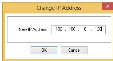
Figure 202. Safety Controller IP Address
