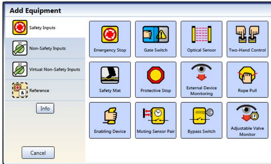
Figure 51. SC10-2: Adding inputs from Equipment View (physical status output can only be added from this view)
