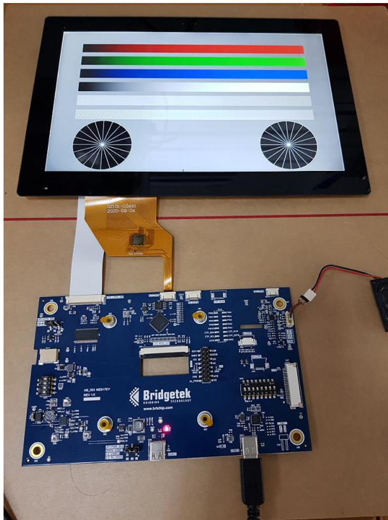
Figure 5-4 - PC setup with 10.1" 1280x800 panel
