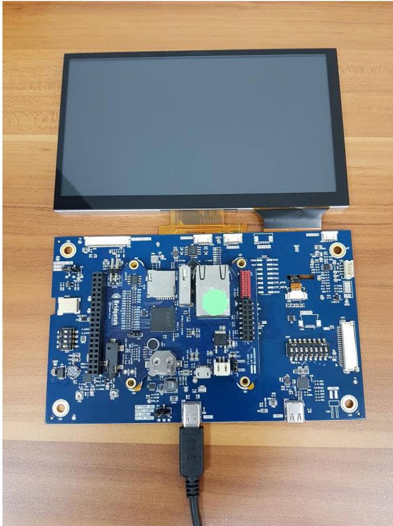
Figure 5-1 – MM900 setup with 7" 1024x600 panel
