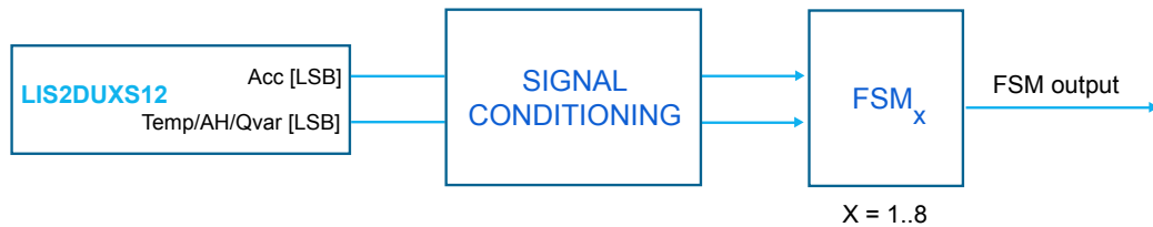
Figure 11. State machine in the LIS2DUXS12
