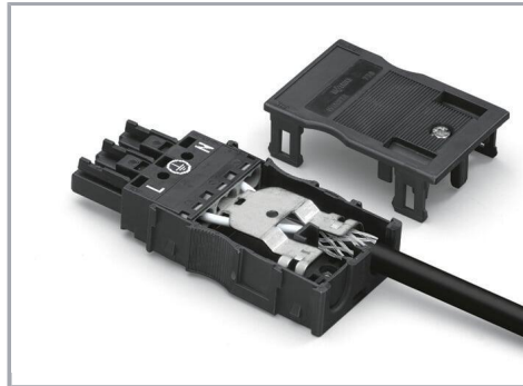
First insert the wired connector into a strain relief housing, then snap cover and tighten screw.
