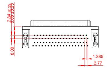
THIS IS A C.A.D. GENERATED DRAWING TOLERANCE UNLESS OTHERWISE SPECIFIED DO NOT MAKE MANUAL REVISIONS TO MASTER. .X ±0.25 .XX ±0.13 .XXX ±0.10
