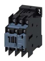
Traction contactor, AC-3 38 A, 18.5 kW / 400 V with solid-state operating mechanism 24 V DC, 0.7-1.25\* Us with integrated varistor 3-pole, size S0 ring cable lug connection
