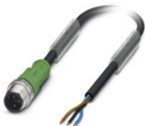
Sensor/actuator cable, 3-position, PUR halogen-free, black-gray RAL 7021, Plug straight M12, A-coded, on free cable end, cable length: 20 m
