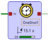
Figure 116. One Shot Block—XS/SC26 FID 4 or later Base Controllers only
