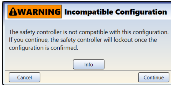
Figure 64. Incompatible Controller Warning
