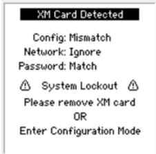
Figure 319. XS/SC26-2d Models: System Lockout
