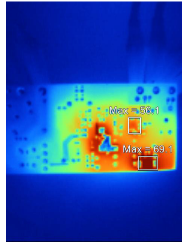
Figure 32. Temperature Checking on Bottom Side, Full Load, 230 Vac
