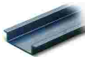
Item no.: 210-196 Aluminum carrier rail; 35 x 8.2 mm; 1.6 mm thick; 2 m long; unslotted; similar to EN 60715; silver-colored
