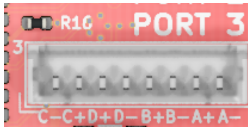
Figure 6: Ethernet port pinout
