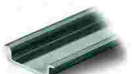
Item no.: 210-505 Steel carrier rail; 35 x 7.5 mm; 1 mm thick; 2 m long; unslotted; galvanized; according to EN 60715; silver-colored
