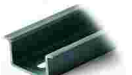
Item no.: 210-197 Steel carrier rail; 35 x 15 mm; 1.5 mm thick; 2 m long; slotted; similar to EN 60715; silver-colored
