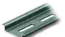
Item no.: 210-504 Steel carrier rail; 35 x 7.5 mm; 1 mm thick; 2 m long; slotted; galvanized; according to EN 60715; silver-colored
