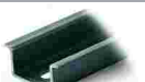
Item no.: 210-508 Steel carrier rail; 35 x 15 mm; 1.5 mm thick; 2 m long; slotted; galvanized; similar to EN 60715; silver-colored
