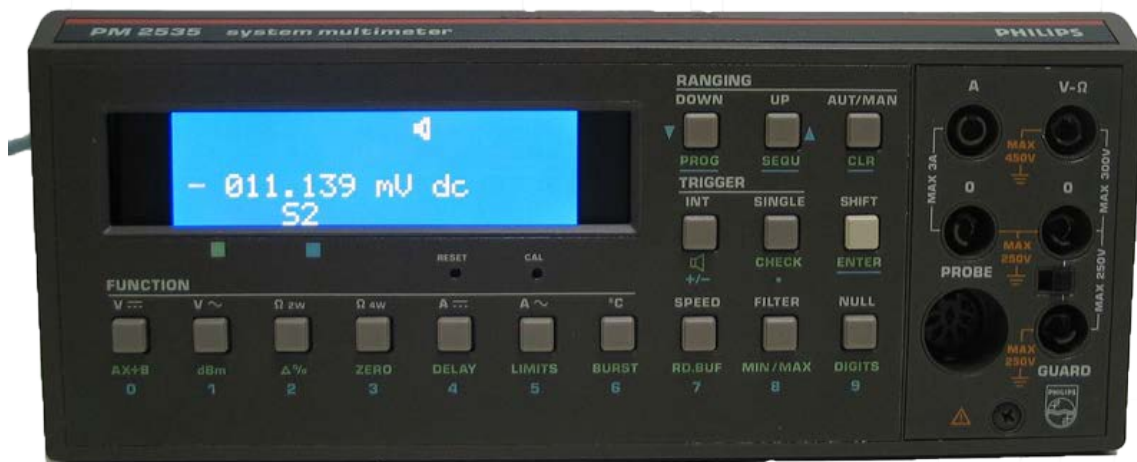
Figure 5. The meter with the repaired display.
