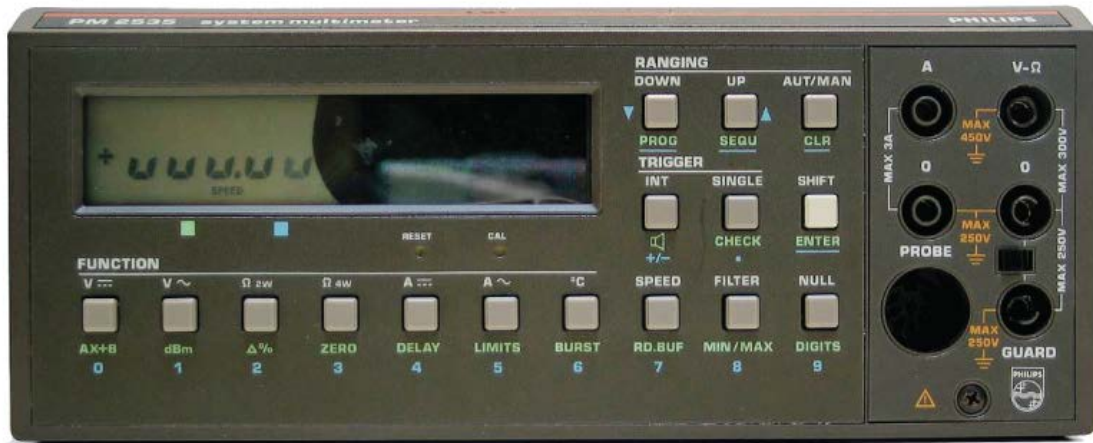
Figure 4. The meter with the defective display, which was beyond repair.
