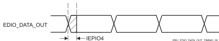
Figure 7-61. PRU-ICSS IEP Digital IOs Timing Requirements
