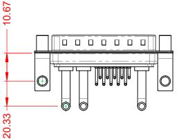
30A (CURRENT) POWER/CO-AX CONTACT RATING: (IF PRESENT) SIGNAL CONTACT CURRENT RATING: 5A PER CONTACT SIGNAL CONTACT RESISTANCE:  $10m\Omega$  MAX. **INSULATOR RESISTANCE:** 5000MΩ min.
